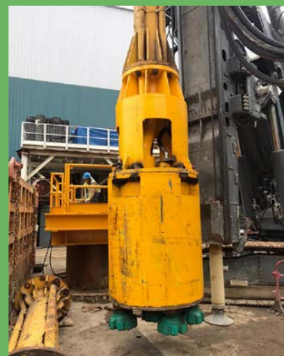
Our cluster bit is ultimately more efficient and requires less diesel than RCD.
